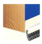
Brush draught excluders are available in various standard lengths from 914mm to 3000mm in aluminium carriers with polypropylene bushes ranging from 12mm to 50mm.
