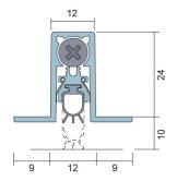
Slim line automatic threshold seal with high efficiency mechanism lifts the seal clear of the floor as soon as the door is opened by a few millimetres.
