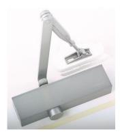
Overhead rack and pinion door closer for light internal doors, for standard mounting, for left and right handed doors up to 1100mm wide. A mounting plate is available for doors where direct mounting is not possible.
