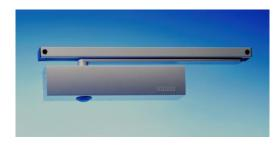
Surface mounted eccentric rack and pinion door closer with guide rail arm for doors up to 1400mm, with adjustable closing force, optical strength indicator, back check, hydraulic latching action and eccentric rack and pinion for easier opening. All adjustments on the front of the mechanism.
