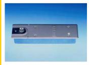
Floor spring for interior single and double action doors up to 1250mm wide with flat cone spindle, adjustable closing force, back check, selectable hold-open and galvanised steel concrete box.
