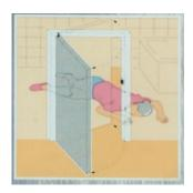
Pivot sets are the ideal solution when fitting toilet doors off restricted areas. The door can be normally opened inwards but in an emergency the door can be easily opened outward by releasing the emergency door stop to gain access.
