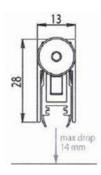
Morticed drop seal to suit 44 or 54mm thick doors Slim line automatic threshold seal with high efficiency mechanism lifts the seal clear of the floor as soon as the door is opened by a few millimetres.
